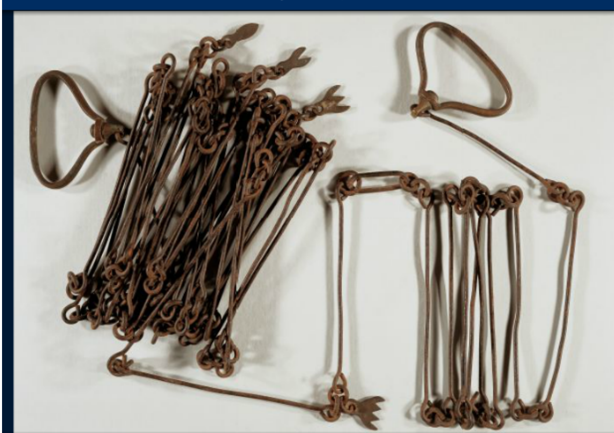
Surveyor's Chain. Lewis purchased this for $2.00. It was used to measure land.
